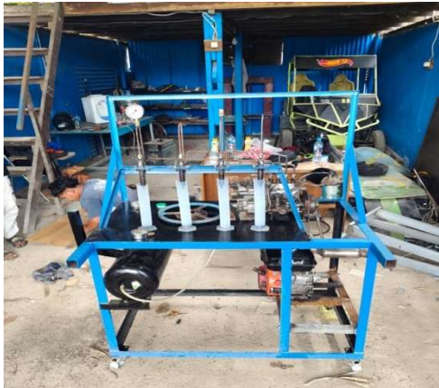
Gambar 3. Rangka Trainer Sistem Bahan Bakar Motor Diesel Tipe In Line
