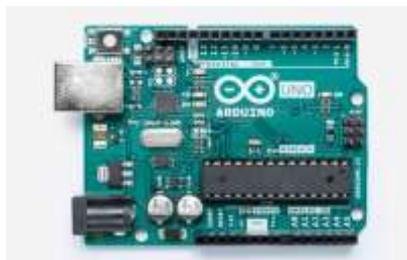
Gambar 2.1 Board Arduino Uno
