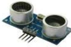
Gambar 2.2 Sensor Ultrasonik
