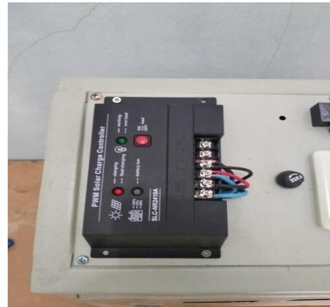
**Gambar 2.3** Solar Charge Controller
