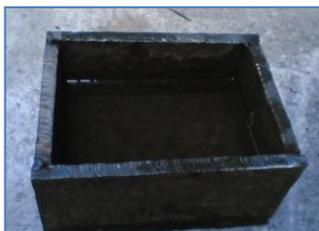
Gambar 29. Housing gear box
