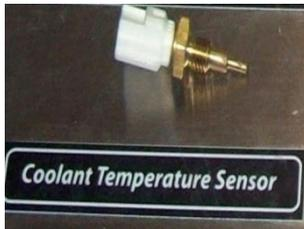
Gambar 4. Coolant/oli Temperature Sensor
