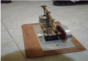
Gambar 5. Model Mesin Stirling Tipe Alpha
