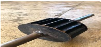
Gambar 7. Turbin Cross-Flow
